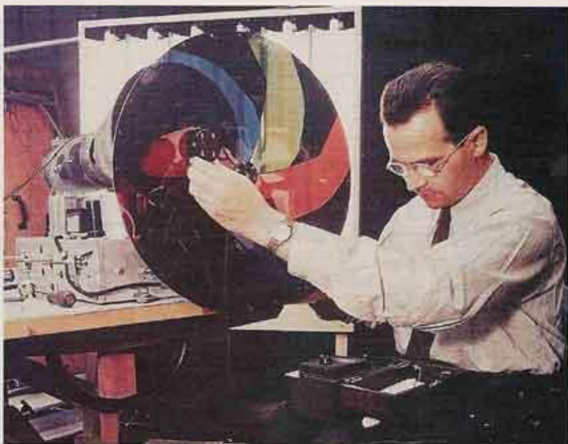
Peter Goldmark of CBS and his color wheel, with its sets of red, blue, and green filters.
