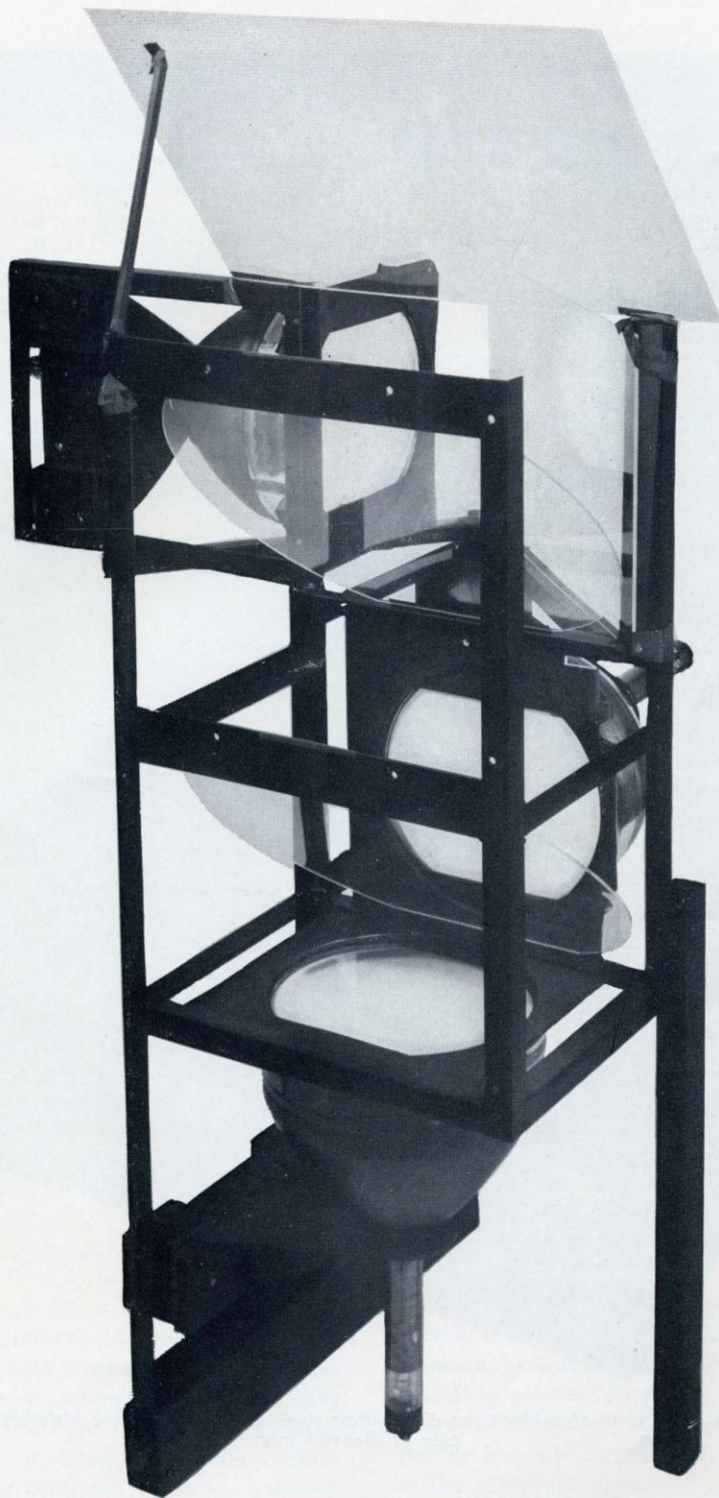
Fig. 9—Positioning of ten-inch kinescopes for direct-view picture-reproducing system.
