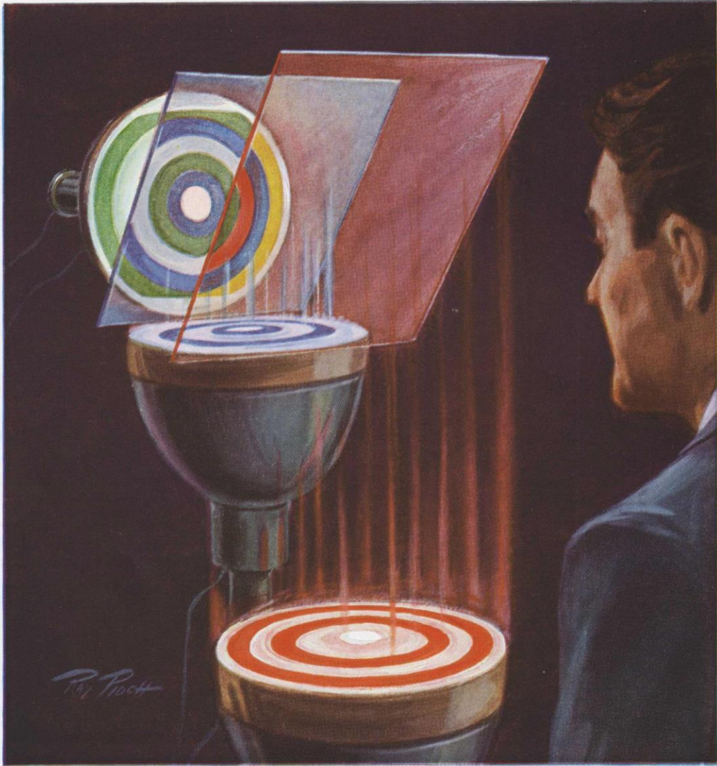
Fig. 8—Direct-view picture-reproducing system using three kinescopes and a pair of dichroic mirrors.
