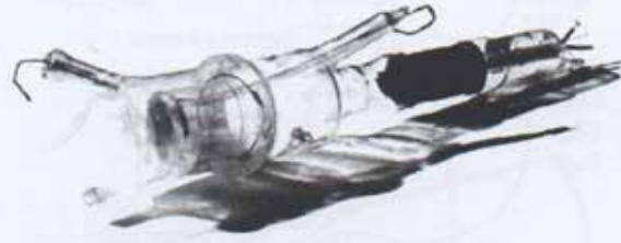
Figure 2.3: Zworykin's first camera tube
