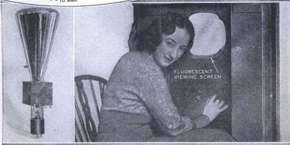
Elimination of the cumbersome scanning disc and other moving parts is made possible by use of the cathode ray tube, shown at left. Image is built up on the fluorescent screen by "pencil" of electrons, which are caused to swing rapidly over screen by electrostatic action of the condenser plates. At right is shown cathode ray receiver used to pick up programs from W6XAO, Los Angeles, California, now broadcasting regularly on 6¼ meters, or 44,500 kilocycles.
