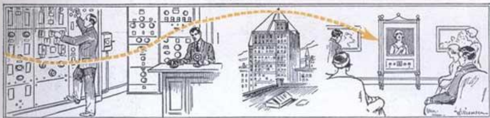
Continuing the path of the television program. The outgoing signal is adjusted in the control and made ready to put on the air over antenna at wave lengths usually around 150 meters. Signal is then picked up at home antenna and led into home television receiver for entertainment of the family. Voice and picture are reproduced in synchronism.
