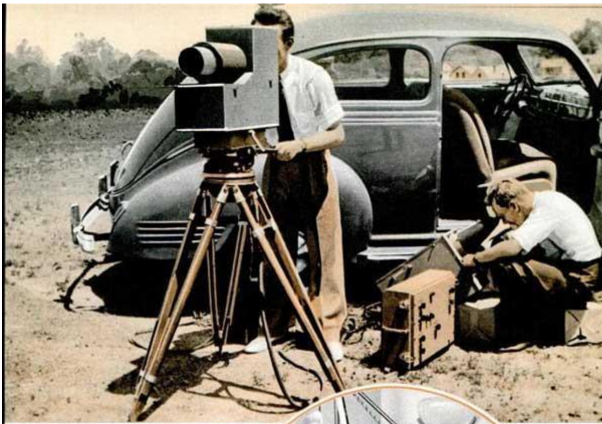
Du Mont television equipment—camera, controls, synchronizing signal generator, power supply and other units—all capable of being packed into auto (above) and (right) applying anode coating to television receiving tube at General Electric.
