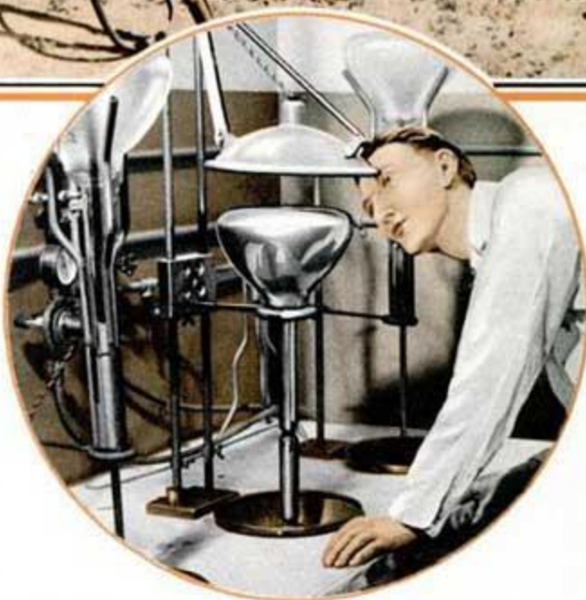
Du Mont television equipment—camera, controls, synchronizing signal generator, power supply and other units—all capable of being packed into auto (above) and (right) applying anode coating to television receiving tube at General Electric.
