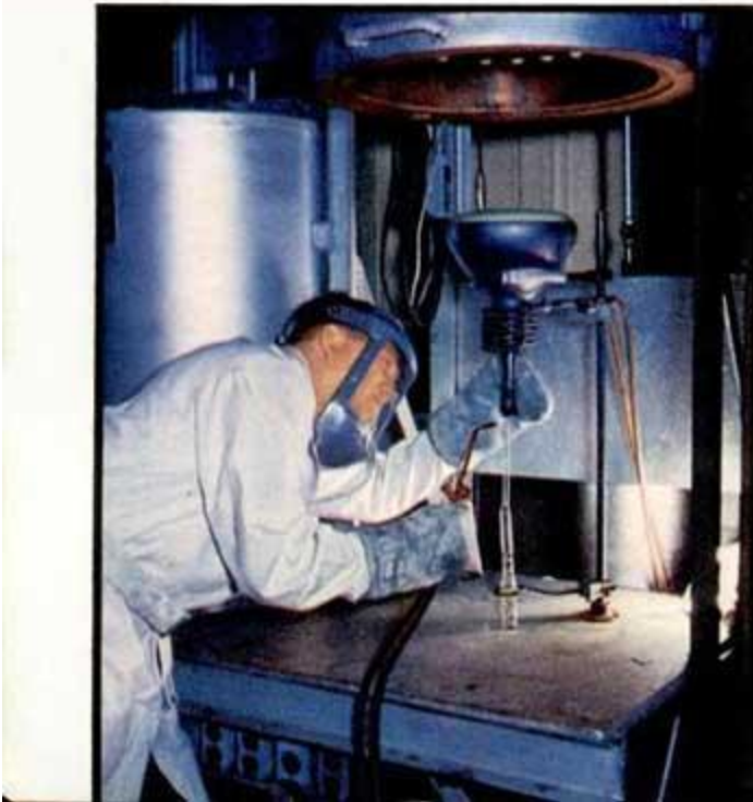
Above, at the controls in General Electric's television studio. This is a natural-color photo, as is the one below which shows a tester applying voltage to television receiving tube. The mask is protection against tube explosion.
