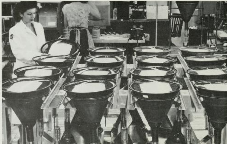
Tri-color TV kinescopes are inspected during a pilot-production run at RCA's tube plant, Lancaster, Pennsylvania.
