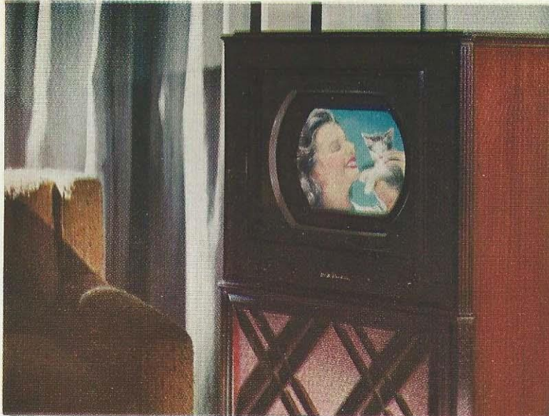
Figure 3b. Development Model Color Television Receiver with an RCA 16-inch Color Television Tube
