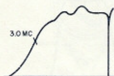
Figure 33—Video Response at 1st Video Amplifier
