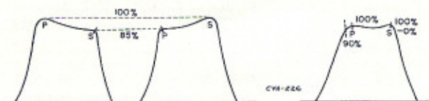
Figure 29—Tuner VHF R-F Response
