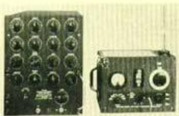
Fig. 5. High frequency signal generator (right) and Phasmaxjector (Monoscope)
