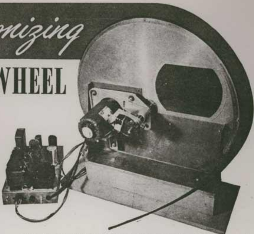
Fig. 1. Color converter with motor control, saturable reactor, and alternator.
