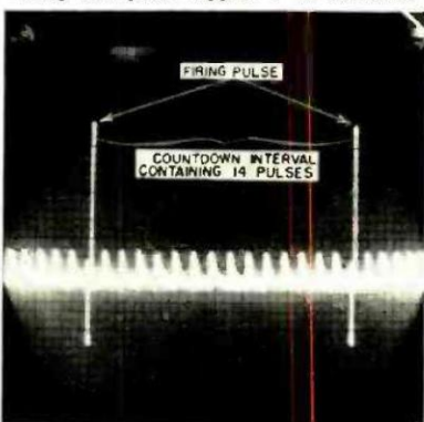
Fig. 11. "Divided by 15" counter pulses on scope when connected to "Test Plug +15". Every 15th pulse triggers ÷15 oscillator.
