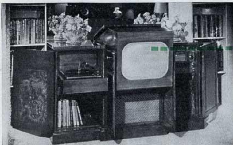
20-INCH screen of $2,495 Dumont set is largest direct-view size. Screen measures 12\frac{1}{8} by 17\frac{1}{8} . Note relative sizes of 10" and 20" tubes in picture at right.
