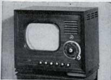
$695 Dumont 15" set has screen about 9½ by 12¾. Its tube weighs 37 pounds.
