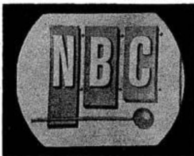
Black-and-white station identification pattern with vertical color stripe imposed (at right).
