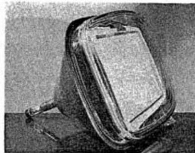
Model of single-gun color crt made by Thomas.
