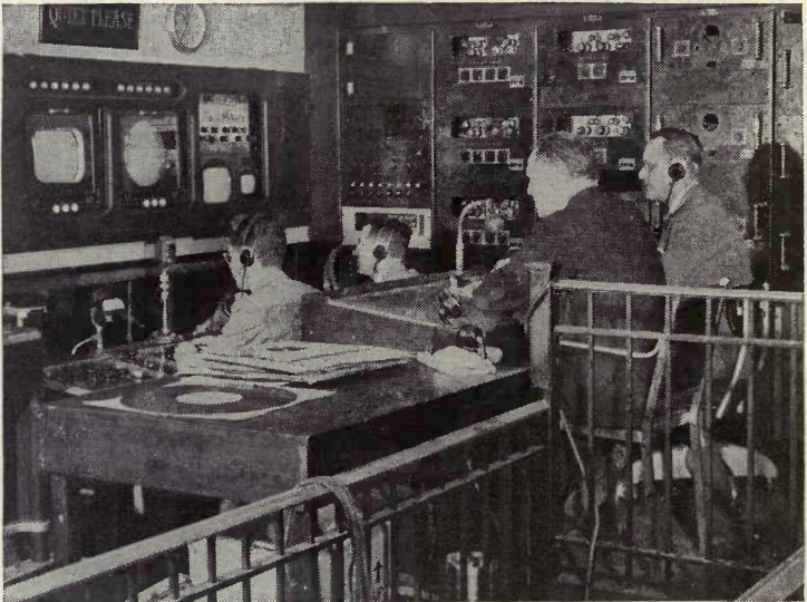
FIG. 14.—A close-up picture of the interior of NBC Television's control room. Sitting at the controls in the left-hand side of the picture are (left) audio engineer and (right) video engineer. Behind them are (left) technical director who is in direct communication with all the technicians and engineers on the floor and (right) producer-director who is in charge of the entire production. ( NBC Television, WNBT, New York. )
