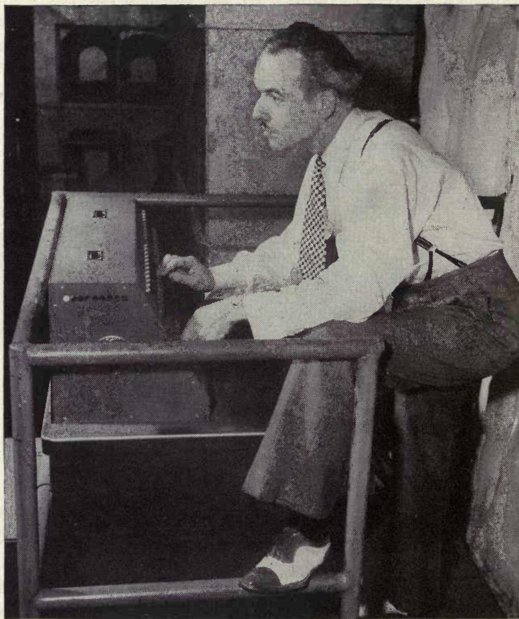
FIG. 37.—Light bridge in studio of WRGB, General Electric's television station. From here by means of push buttons, the ceiling mercury-vapor lamps are turned off or on, tipped or tilted in any preferred position. ( General Electric Company. )
