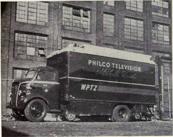
FIG. 101.—Mobile unit of Philco television station WPTZ, Philadelphia, ready at all times to transport the remote pickup television cameras and equipment to the scene to be televised. ( Philco Corporation. )
