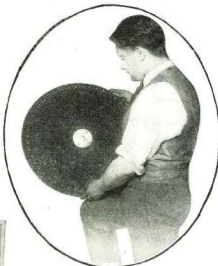
The disc whose size is shown at the center has small square holes through the larger white dots, which are the aluminum exposed. (Courtesy of Lexington Television Corp.) Below, the arrangement of the set-up: 1, neon-lamp plate; 2, base support; 3, driving mechanism; 4, rheostat; 5, hood.
