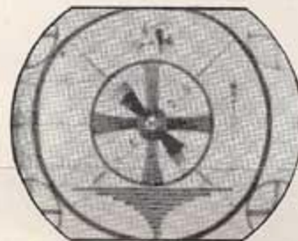
Figure 8. Improper focus; adjust FOCUS.
