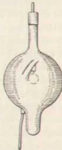
FIG. 170.— Photo-electric cell for tele- vision projec- tor.
