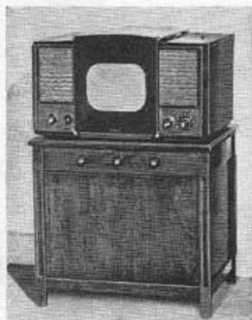
Figure 1. Front view of the complete Duo-Vue conversion unit with television receiver attached
