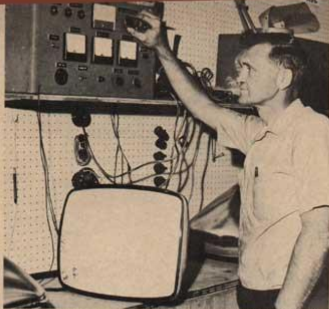
Bud checks a rebuilt tube on his special test unit which indicates emission, shorts, leakage and gas content.
