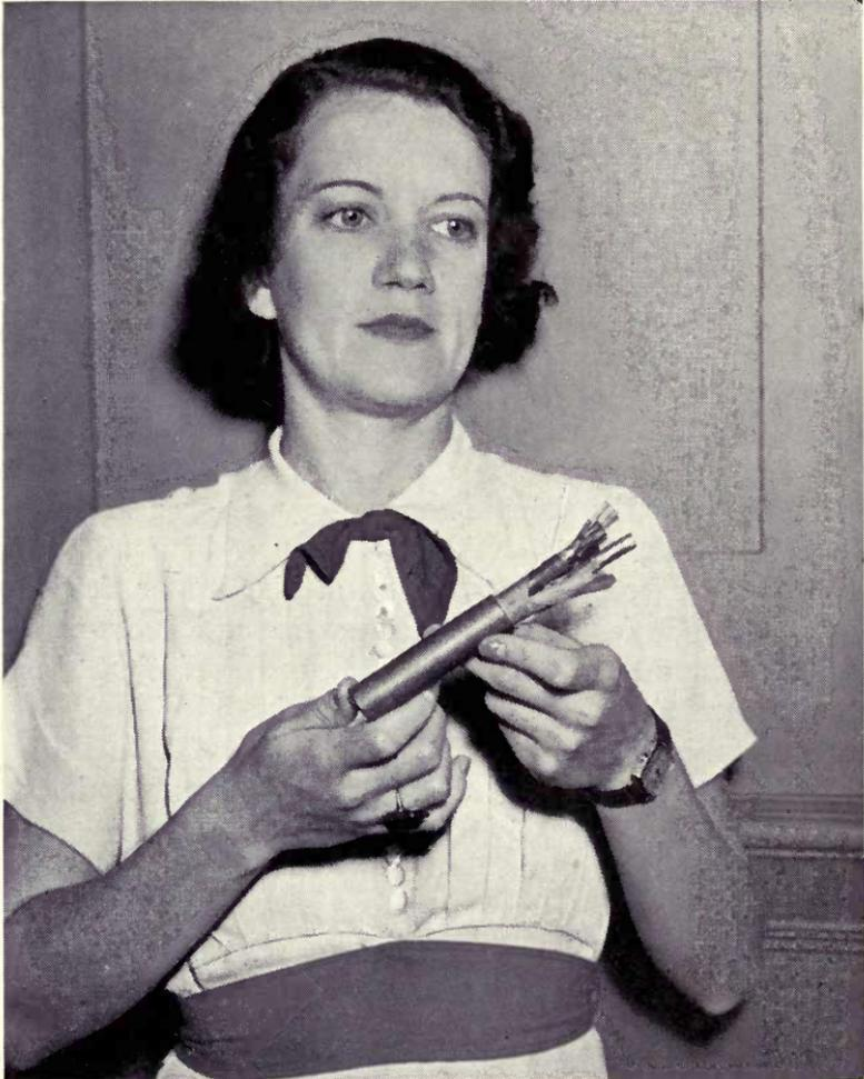
Fig. 44. Piece of Co-axial Cable. The two large tubes can be used for television circuits and the eight other wires are for signaling and control circuits
