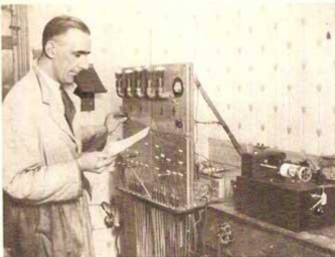
ABOVE: Mr Gilbert Miles operating a facsimile device for transmitting pictures by radio, developed by Television and Radio Laboratories Pty. Ltd.
