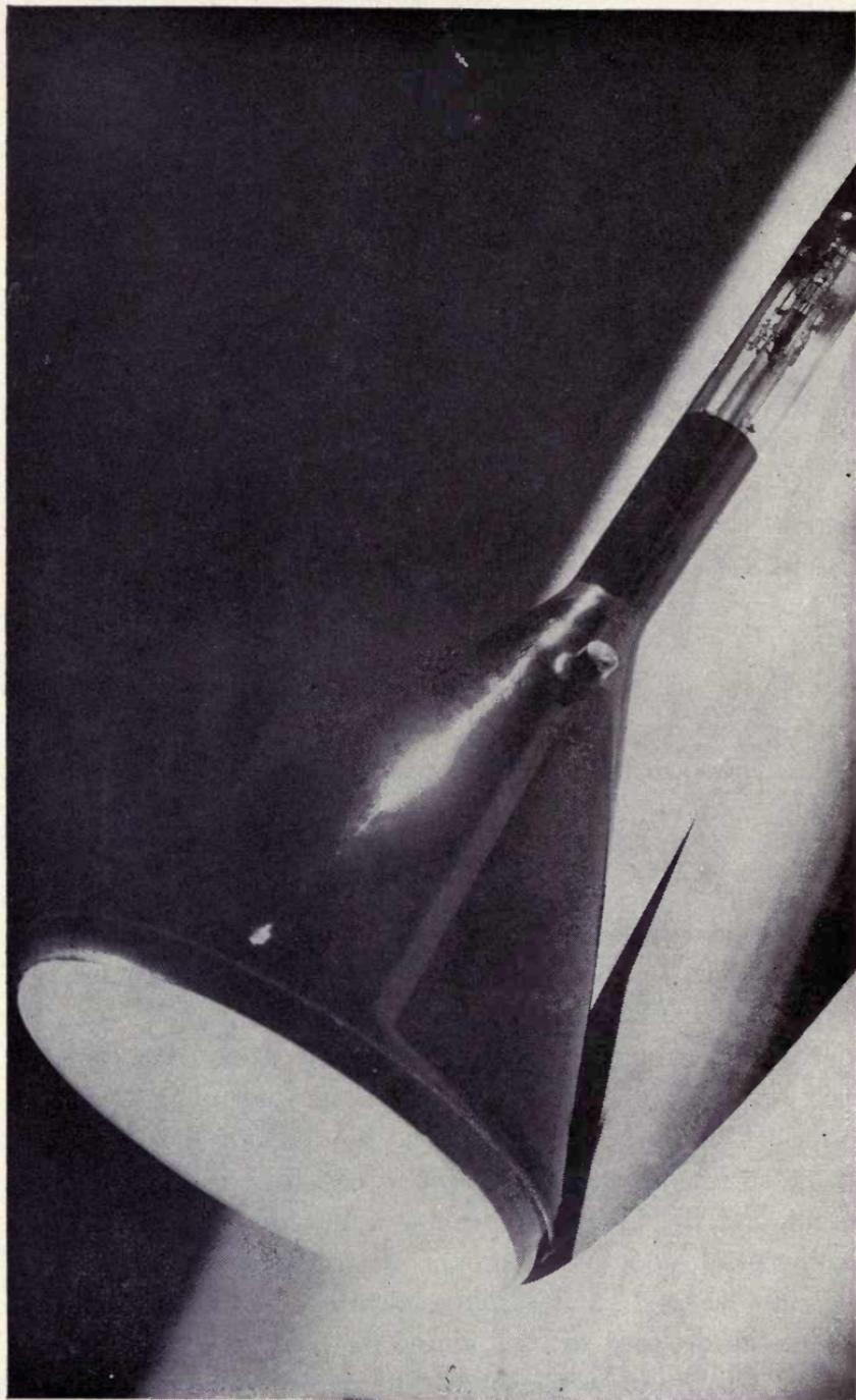
THE CATHODE-RAY VACUUM TUBE — OR KINESCOPE
