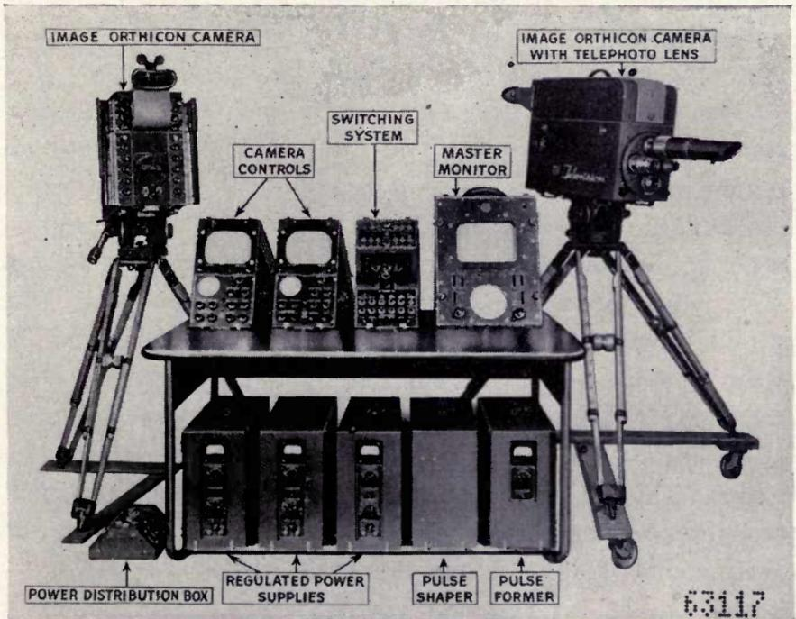
NECESSARY BASIC STATION EQUIPMENT FOR REMOTE PICK-UPS
