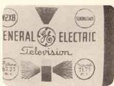
FIG. 14. INCORRECT SETTING OF HORIZONTAL CENTERING CONTROL
