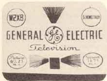
FIG. 8. INCORRECT SETTING OF VERTICAL LINEARITY CONTROL
