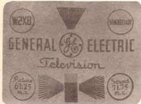
FIG. 4. EXCESSIVE CONTRAST, LOW BRIGHTNESS
