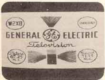
FIG. 10. INCORRECT SETTING OF VERTICAL SIZE CONTROL
