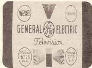
FIG. 13. INCORRECT SETTING OF HORIZONTAL SIZE CONTROL
