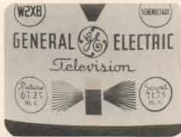
FIG. 9. INCORRECT SETTING OF VERTICAL CENTERING CONTROL
