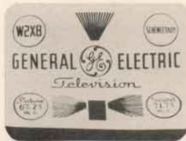
FIG. 10. INCORRECT SETTING OF VERTICAL LINEARITY CONTROL
