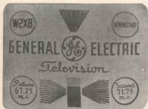
FIG. 4. EXCESSIVE CONTRAST, LOW BRIGHTNESS
