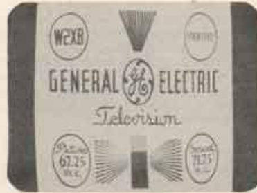
FIG. 11. INCORRECT SETTING OF WIDTH CONTROL
