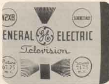
FIG. 8. INCORRECT SETTING OF HORIZONTAL CENTERING CONTROL
