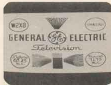
FIG. 14. INCORRECT SETTING OF HEIGHT CONTROL
