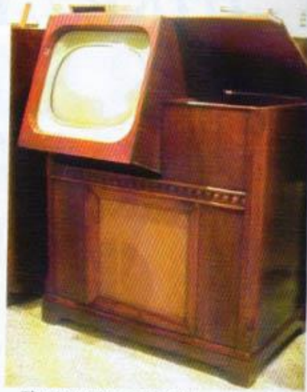
The 1949 Emerson 608 has a 16-inch screen. The picture tube tilts into the cabinet when not in use.
