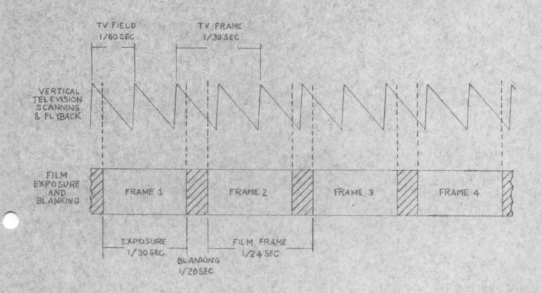
Figure 3-8. Time Relationships Between Scan and Film Exposure
