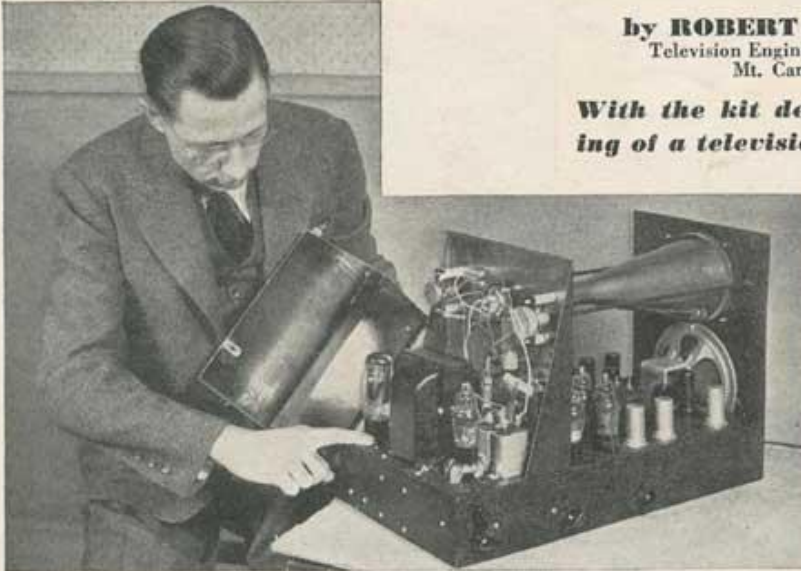
With the power circuits completely enclosed, the safety factor is greatly raised.
