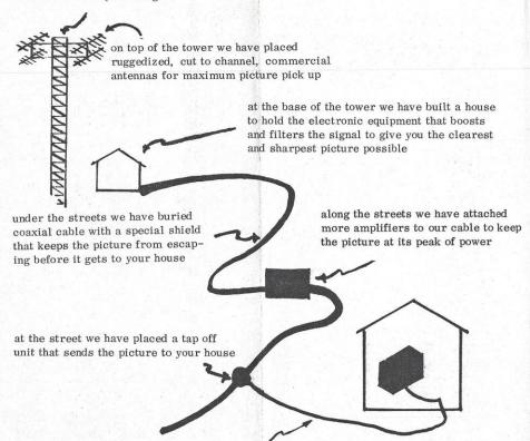
the cable runs underground (no ugly overhead wires) to your house and can enter the house through the same place as your present lead in wire and connect to the back of your tv set (no ugly antenna on your roof)
