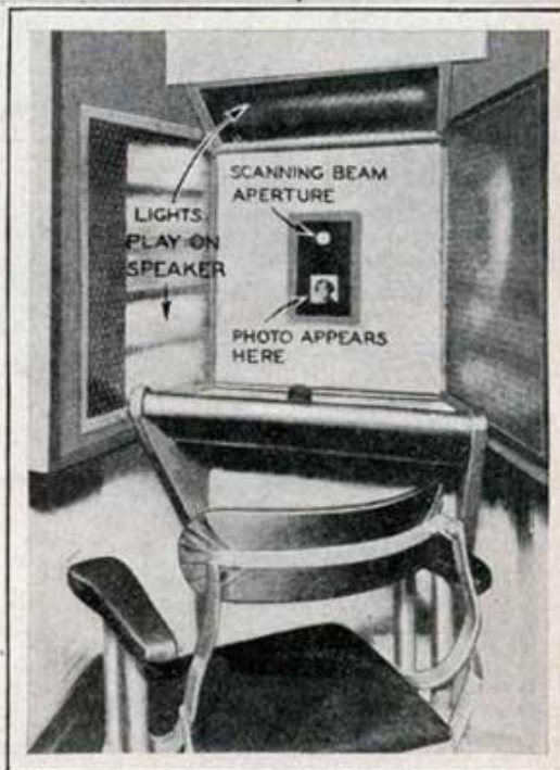
Above: A diagrammatic sketch of the combined radio and television apparatus. The voices and images of the speakers are being transmitted simultaneously. Below: Booth with the photo-electric cell lights which pick up the man's image, and the reproducing screen.
