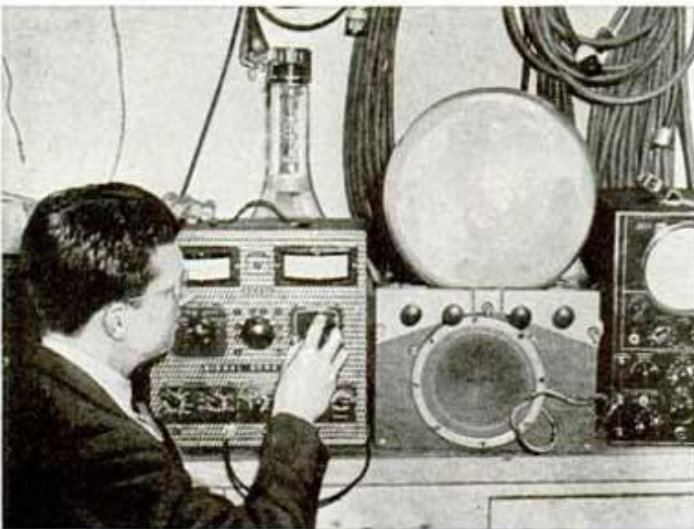
Testing a television receiver by means of a signal generator and a cathode ray oscillograph in laboratory at station W6XYZ
