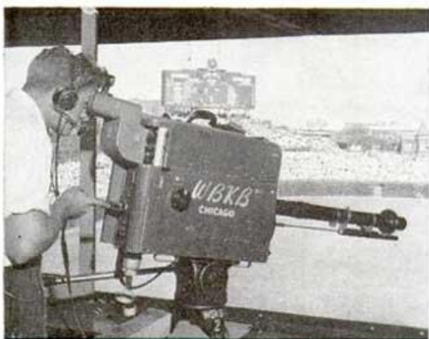
At Wrigley Field in Chicago, cameraman gives his Zoomar lens a pregame test. By manipulating lever he can change focus for a close-up of ball or wide-angle shot of field
