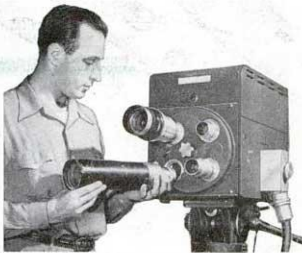
Camera's turret mounts four different types of lenses. Cameraman can change from one lens to another by manipulating the controls
