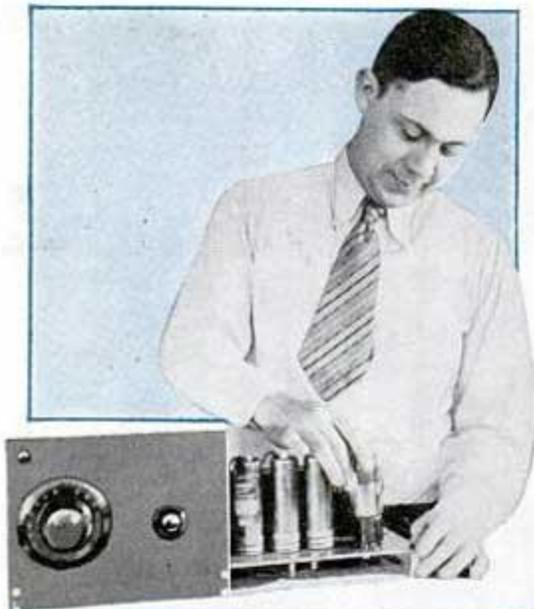
and also requires but one adjustment. All fixed resistors are of the 2-watt type and should be of the best quality obtainable. The optional .5-mfd. by-pass condenser should be used if motor-boating is encountered, and the .001-mfd. will be found very helpful in many cases.
