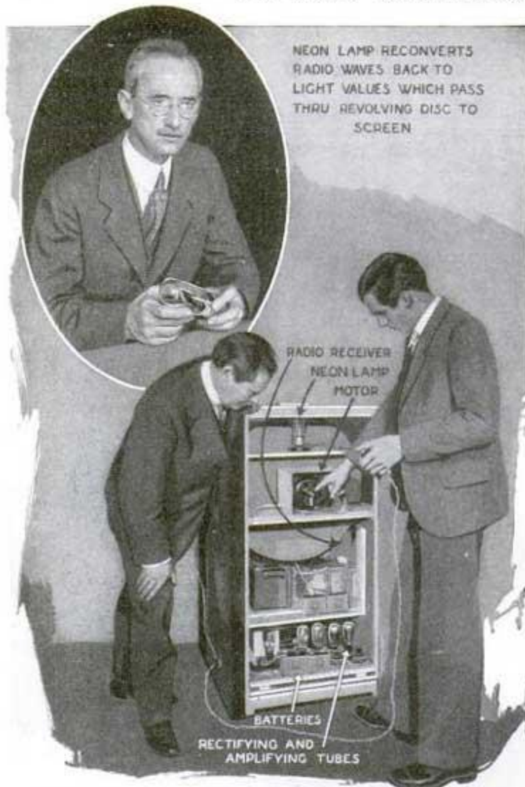
The Motor-Driven Pinhole Disk, the Neon Lamp That Reproduces the Image and the Picture Receiver
