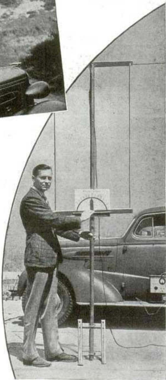
Device used in the field to measure the wave that carries the television image
