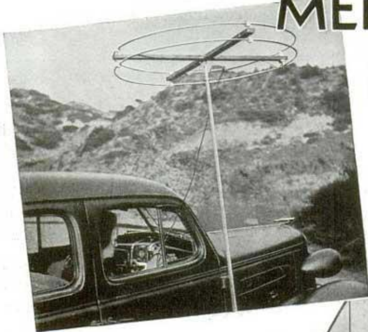
Directional antenna for a television receiver installed in an automobile. Amateurs contribute much with experimental work
