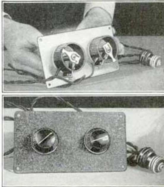
Rear View of Television-Motor Control Ready for Mounting, and, Front View Showing Control Knobs
