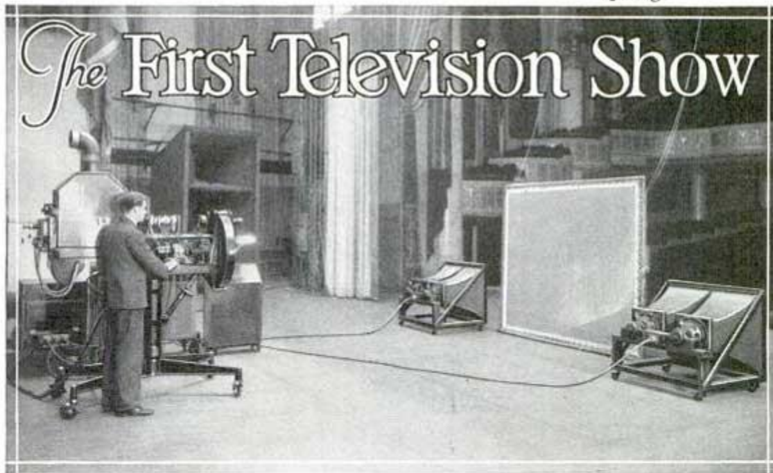
R. D. Kell, Operating Television Theater Projector. Showing How the Picture Is Projected from Back-stage; beside the Screen Are Loud Speakers for Reproducing Accompanying Radio Voice
