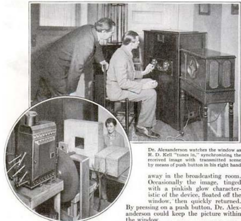
Television transmitter, showing arc light holder, perforated disk and lens casting rays on subject.
