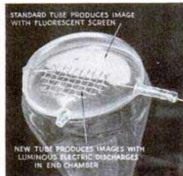
Close-up of combination window in model of new tube, built to contrast the brightness of projected image of the old and new types
