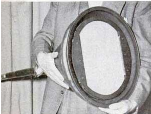
The one-gun, tri-color tube looks like this. RCA engineers are working on improved models, with more dots. Tube can be used in some standard receivers, but needs extra circuits.
