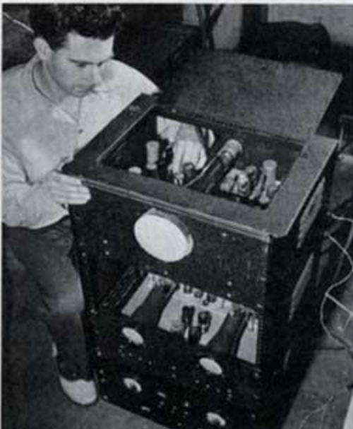
Control assembly started as a single oscillator. It develops three sets of synchronized signals that form the composite signal or picture.
