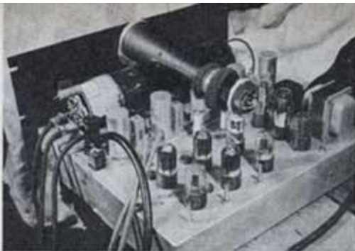
Lovely Gwendolyn reposes in lightproof tube made from candy container. On top is a monitor scope; in the foreground is the timing unit.
