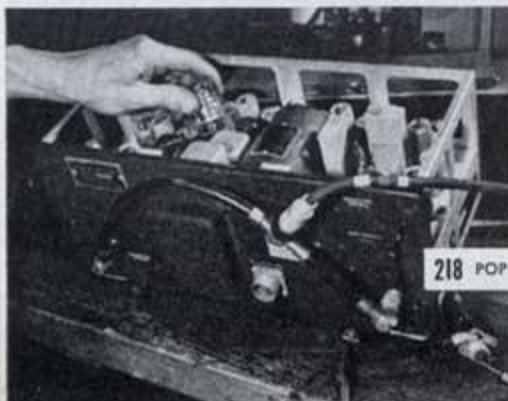
Radio altimeter is used to convert a standard receiver to pick up the 429-mc. experimental band on which the broadcasts go out.
