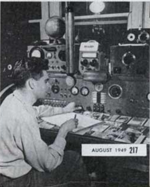
Voice accompanies the picture. This is the control console of W6JDI-TV; it serves also for regular transmissions on other ham bands.
