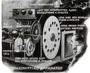
In the transmitter rotating disks divide the face into patches of light of varying intensity. These the photo-electric cell translates into correspondingly fluctuating electric current
