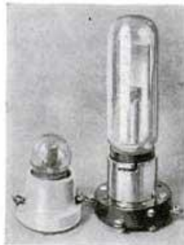
Fig. 3. Left: Small neon tube that can be used for television. Right: Large neon tube specially designed for television.
