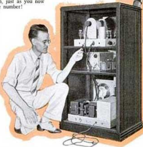
Workmen installing a lightning arrester to protect the antennas of a television station in the Empire State Building, New York City. Left, a modern television receiver with sight and sound circuits housed in a single cabinet
