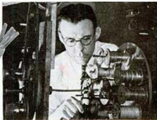
A NEW AID FOR RADIO ENGINEERS A part of the intricate machine that winds the "coaxial" cable which can carry 200 telephone calls at once. Left, a section of the cable showing its twin copper tubes and eight wires
