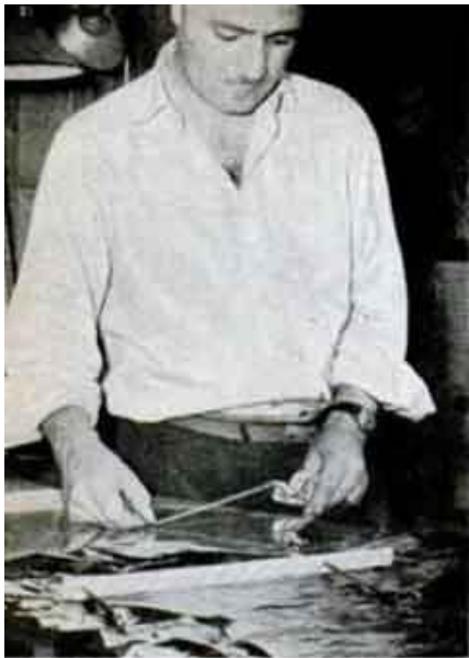
Making the wheel. I started with a 21" square of Lucite 1/16" thick. After sawing it to a rough circle, I centered it on the threaded shaft, clamping it between washers and nuts. Then I cut it to a true circle by holding a chisel to the edge while it ran. Cut-outs of colored cellophane, taped to the plastic, completed the wheel.
