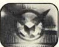
Picture out of focus—Focus control needs adjusting.
