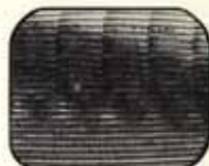
Screen composed of black dashes—Line hold control needs adjusting.
