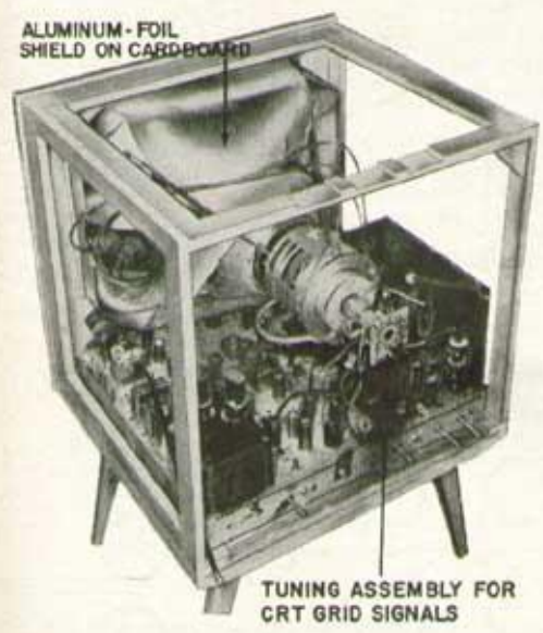
An experimental color receiver using the Apple tube.
