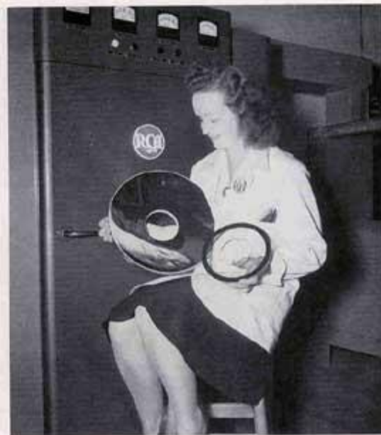
12. The two lenses, completed and ready for mounting in the projection-type home receiver. In the background is the standard RCA Type 15-B Radio Frequency Generator used in preheating the plastic disks before molding. At the right rear is the screened enclosure containing the heating electrodes.
