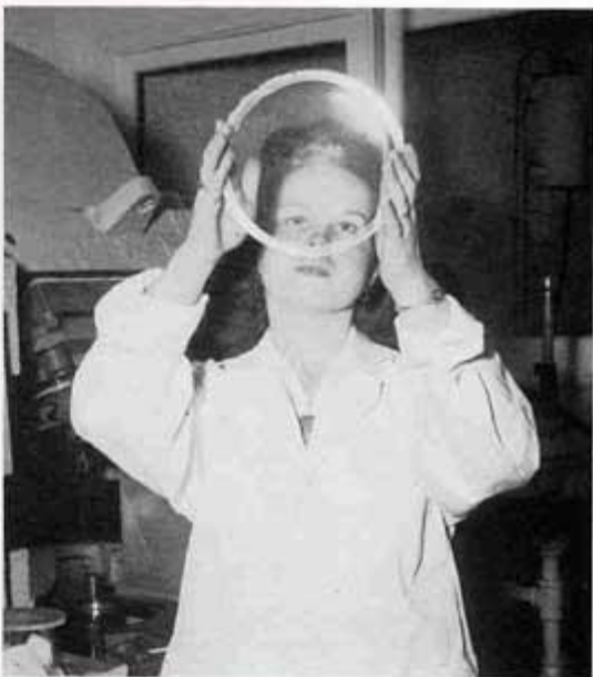
8. Lenses molded in this way have excellent optical properties. They have slightly better light transmission than glass and slightly less light scattering—both of which are, of course, advantageous. They do not have the surface hardness of glass, but in tests have stood up well without any special care.
