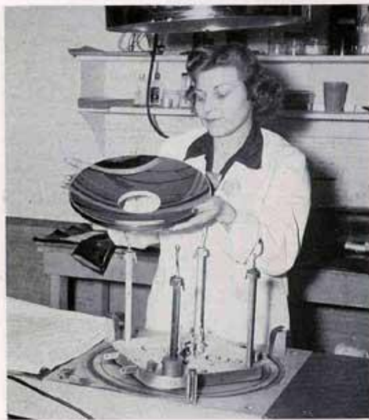
11. The spherical mirror, removed from the bell jar after aluminizing has been completed, is shown in this illustration. The polished, aluminized inner surface has a true "mirror-finish" of high reflective properties. As a "lens" it has very high light gathering power.
