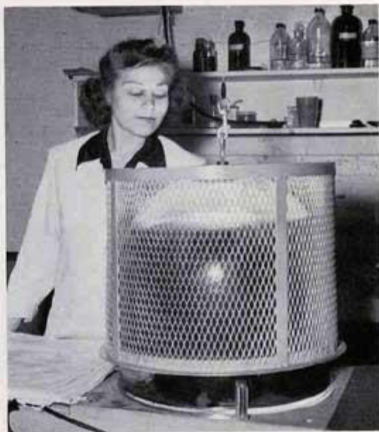
10. The aluminizing procedure consists of placing the glass bowl—inner side down—in a bell jar which is then evacuated. In the jar are two aluminum filaments from which aluminum is evaporated by heating to incandescence. The aluminum vapor which is driven off condenses on the under side of the glass.
