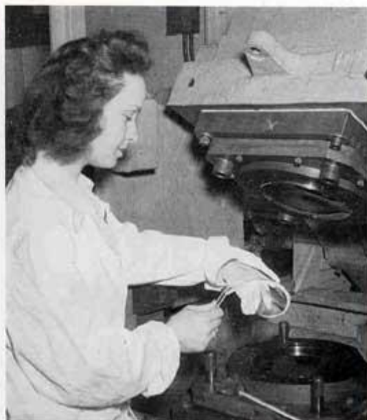
6. The heated disk (usually referred to as a "preform") is soft and flexible as it comes from the radio-frequency preheating cabinet. The molds, heated by steam pipes, keep it soft during pressing. When the heating cycle is completed, steam is shut off and cold water turned on.
