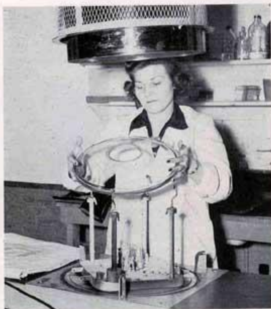
9. The spherical mirror which forms the main "lens" in the reflective optical system is shown here before aluminizing. It is a saucer-bowl shaped piece of glass 14 inches in diameter with a 4-inch hole in the center. The inner surface is ground to a true spherical shape on a standard optical grinding machine.
