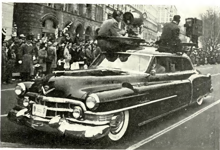
Fig. 6—The Cadillac Telemobile Unit moving down Pennsylvania Avenue toward the White House. The microwave relay dish is aimed at the Capitol.
