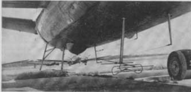
Two 4-element retractable yagis were used beneath the fuselage.
