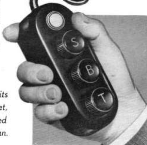
Fig. 1. The Emerson model 1158 remote-control unit shown here is capable of duplicating all of the TV set's front panel adjustments for picture and sound.
