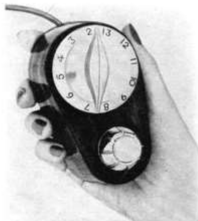
Fig. 3. Channel-selector, "on-off" switch, and volume control are included in this remote-control unit for Walsco TV sets.
